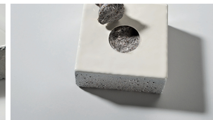
Mode Of failure demonstrates a full concrete failure
